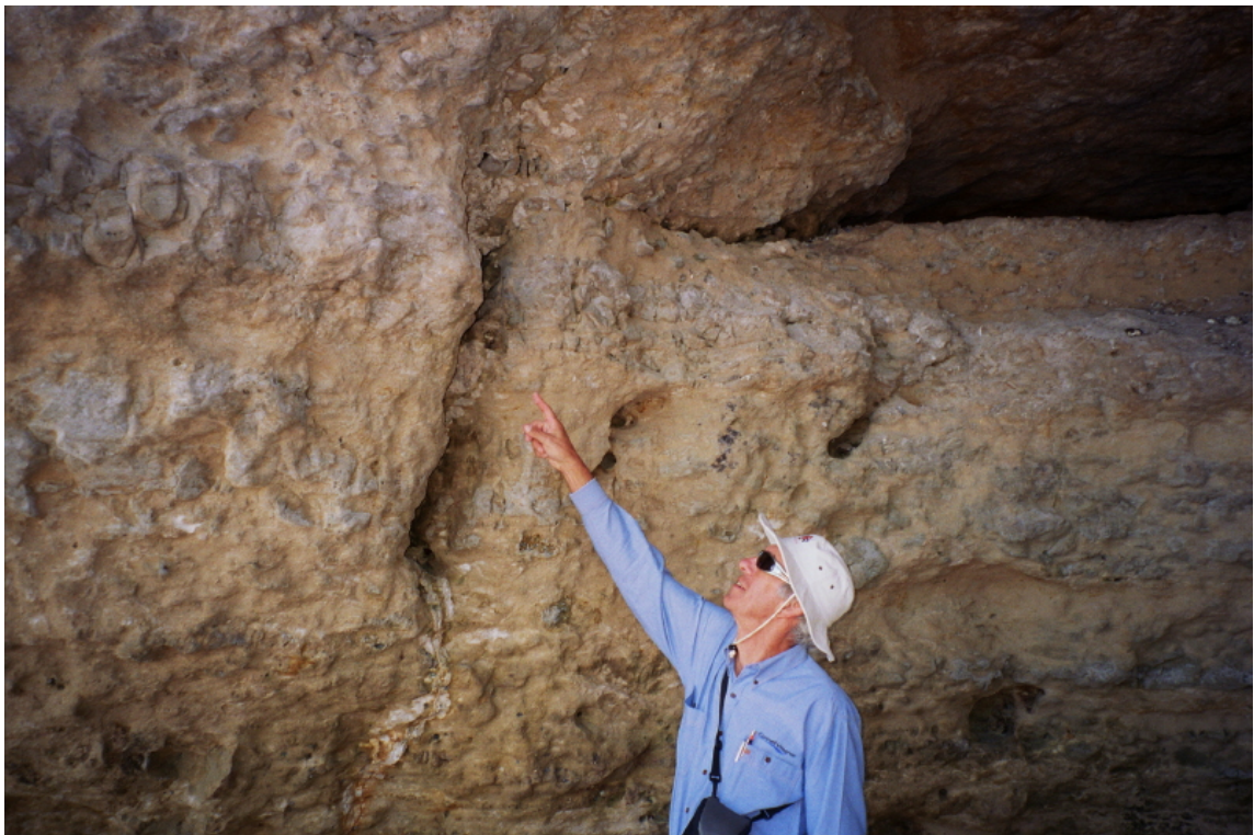
Plate 12 Partly infilled vertical defect providing release surface in the cave from Plate 11
