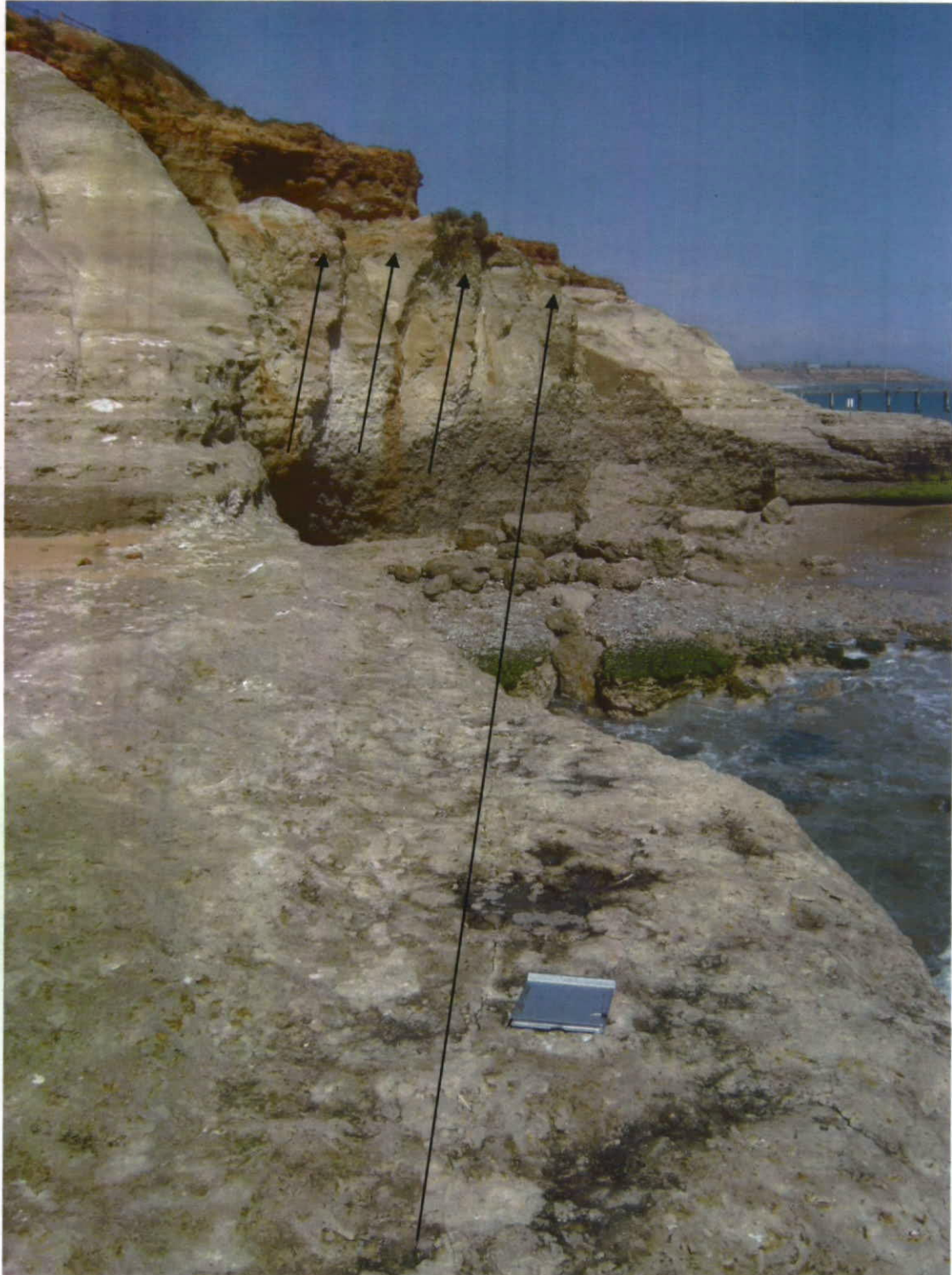
Plate 36: View looking south down onto large boulders that have recently fallen onto the current wave cut platform. In the foreground, left of the silver folder, tension cracks in the rock align with subvertical joints observed in the area where the slope failed (refer to arrows). Note the persistence of these structures is greater than 20 m in length.
