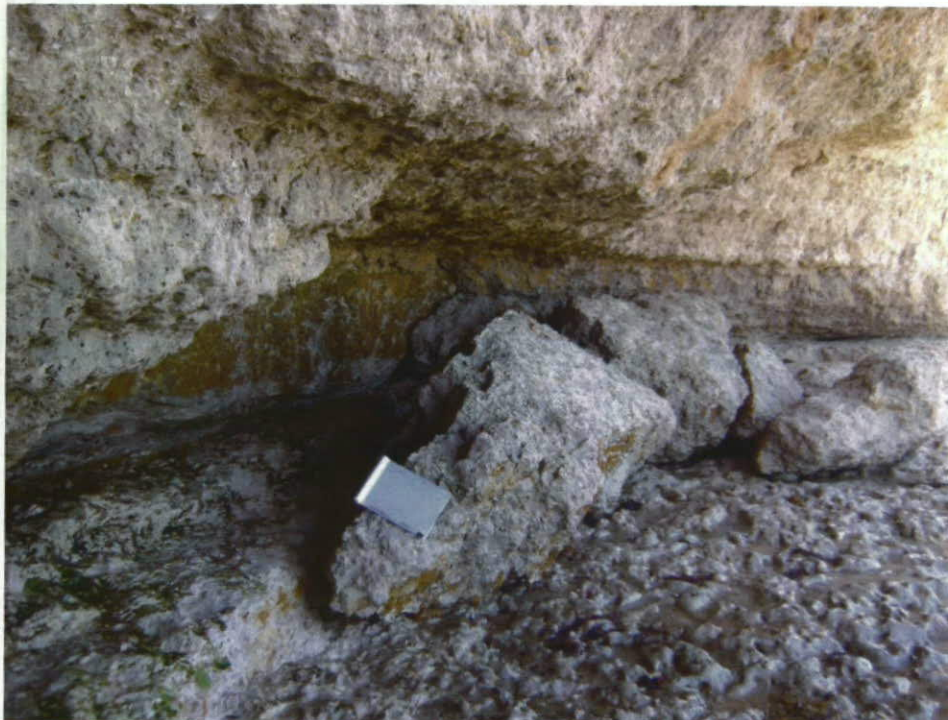
Plate 38: Close up of recent rocks fallen due to the forces of wave action which have undercut the cliff and have formed a cave. Cave depth is >5 m and >10 m in length. Rock failure due to horizontal defects and gravity, leading to tensile failure of the rock mass.
