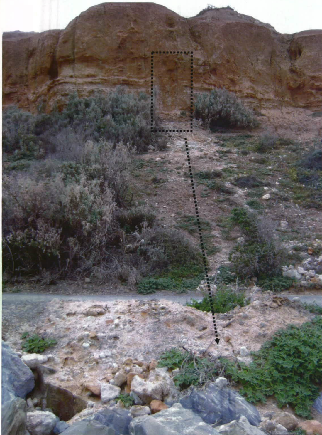
Plate 17: Recent toppling failure of sandy soils from the upper cliff face resulted in shrubs being destroyed and material transported down the slope over the walkway. Failure due to undercutting of cliff and subvertical tension cracks in vertical sandy slopes.
