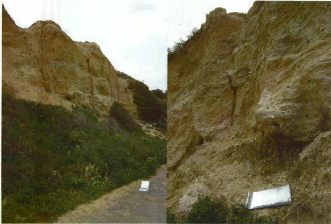
Plate 7: General view of slope on the left and an enlarged photo of the weathering soils on the right. Water erodes gullies in sandy gravelly soils and the undermining of slopes by the dessication of discrete clay layers create potentially unstable subvertical cliffs.
