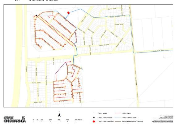
6.7.1 The Sellicks Beach scheme is comprised of two separate residential developments (Prodec and OVE). Prodec is a Septic Tank Effluent Discharge collection system and OVE is a sewer collection system. Wastewater discharges to Sellicks Beach. The scheme services 382 customers (residential only) with \$263,580 income generated in 2017-18.
